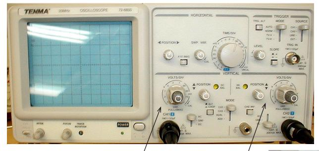
"Dual channel" oscilloscopes like this one can display two different traces in order to compare two signals being measured. They have two VOLTS/DIV controls -one for each channel, that can be calibrated separately. (They will both use the same TIME/DIV setting.) And each can separately be set to display AC, GND (ground), or DC.
