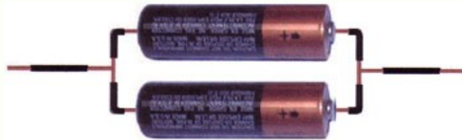
Batteries in parallel.
